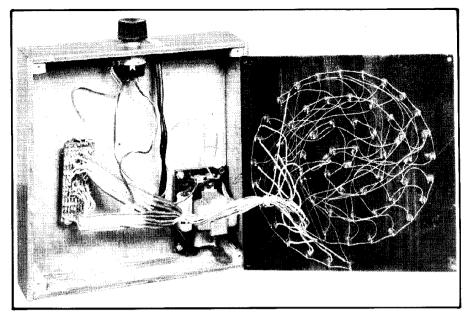
wire switch S1 as shown in figure 3. Use the smallest filament transformer you can find—even at 12 volts the unit only draws 60 milliamperes. *Do not*, however, *exceed 15 volts dc*, or yoù can destroy the ICs. If you use a transformer rated at 6.3 volts at 300 mA, for example, you'll probably find you have 8-9 volts at the output because of the low current drain.
